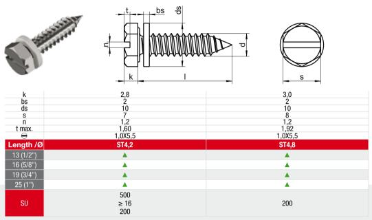
■ A1 / ▲ A2 / ● A4 | SU: Sales units | All measurements in mm / inch | Other dimensions on request. Example item no. 9230-2-4,2X13 WS 9230 - A2 - Ø 4,2mm - I = 13mm
